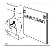
Mount the decor panel by inserting the two pivots of the cross-bar into the slotted holes of the door. Lift the decor panel until perfect alignment with the facia panel is obtained: if the two brackets have also been used, they will automatically enagage in the special holes provided on the dishwasher door.
